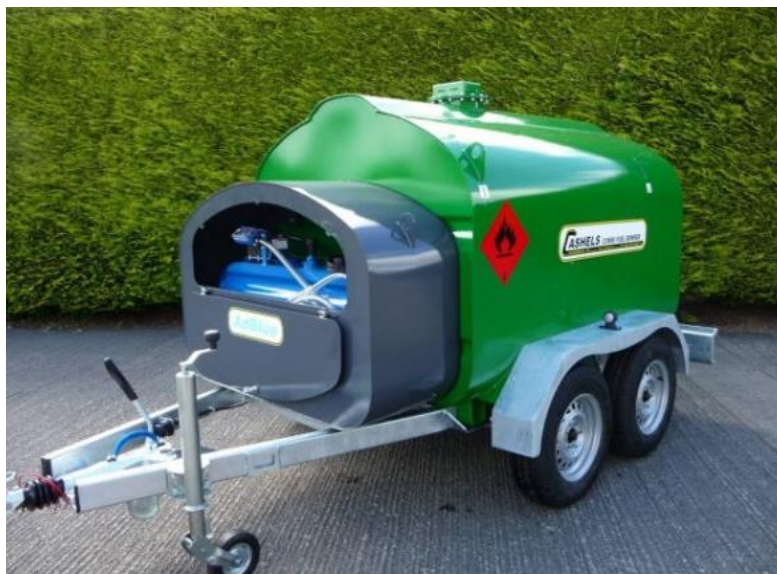
Figure 8.1: Typical mobile fuel bowser (Source: Clarke Machinery Group)
