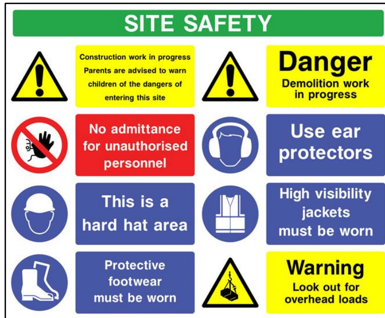
Insert 4.1 – Example of Site Safety Signage
